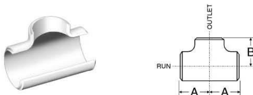
Dimensions (based on ASME/ANSI B16.9) and example weights for equal tees
