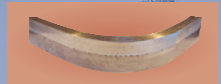
Sidebend test 90° open air cladding (oxide agglomerations are visible)
